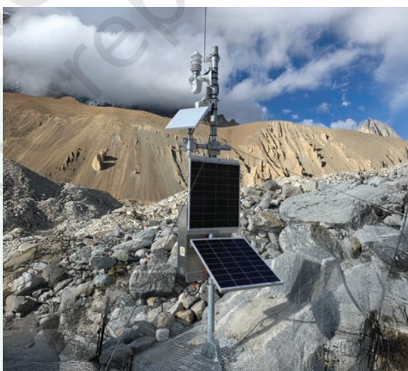
Fig. 2.12. AWS at a glacial lake of Sikkim
